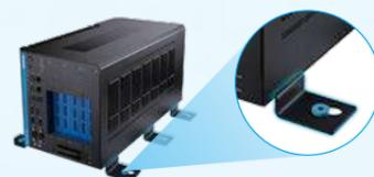
With a robust mechanical design featuring structured support, GPU retainer, cable screw lock, and damping bracket, ASUS IoT edge AI systems excel at in-vehicle situations for smooth and uninterrupted operation.
