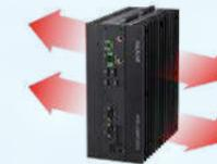
The patented system design effectively diffuses heat from the CPU, GPU and all peripherals, delivering extreme ruggedness with a fanless structure. This ensures stable operation while the fanless design further reduces dust throughput and build-up, enhancing durability.
